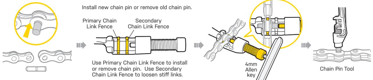
Use Primary Chain Link Fence to install or remove chain pin. Use Secondary Chain Link Fence to loosen stiff links.
