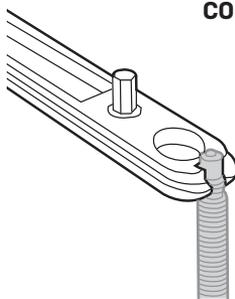
Tighten or remove two-piece Presta valve cores.
