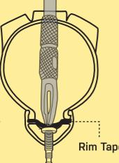
Do not insert the plug tool too deep, otherwise it may puncture the rim tape and cause an air leak
