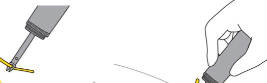
Insert Plug Tool into the puncture with 10 - 15mm of the repair plug ends remaining outside of tire
