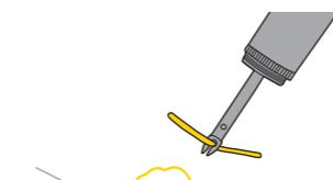
Insert a repair plug through slot of the Plug Tool
