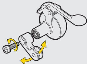
Use 3mm Allen key to loosen bolt and adjust to desired position
