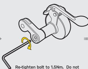
Re-tighten bolt to 1.5Nm. Do not over-tighten.
