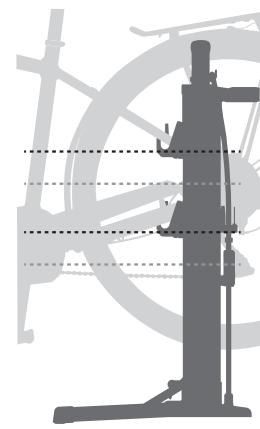
**2** Lift bike onto Hooks then fine tune height adjustment as necessary.
