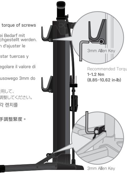
Use 3mm Allen key to adjust the torque of screws if necessary.
