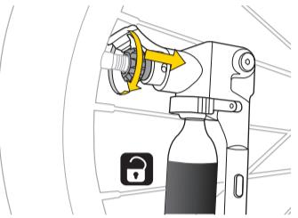
To avoid possible personal injury and damage to bike and/or tool, ensure to disengage CO<sub>2</sub> inflator properly after use by unthreading inflation head in correct direction.
