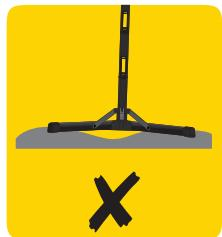
**DO NOT** use on grass, loose dirt, gravel, uneven or soft surfaces. Check the stability of the FLASHSTAND eUP periodically to insure safe storage of your bikes.
